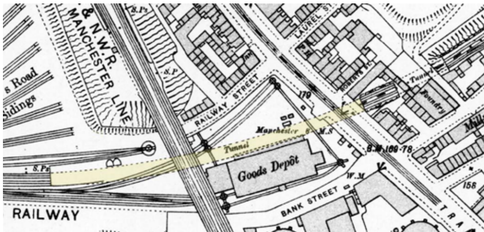
Wellington Road Tunnel is highlighted. The tunnel ran from the George Road sidings, under the LNWR main line and the CLC Wellington Road goods depot. A second shorter tunnel is noted to the east under Wilkinson Road
